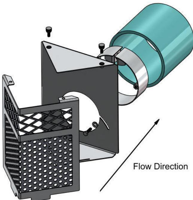
The expanding ring goes into the outlet pipe opening, and allows you to torque a bolt until the ring is tightly secured onto the pipe. Then the back plate can be installed onto the expanding ring and the front cover be placed on and secured with two thumb screws. The expanding ring requires no power tools or drilling of existing structures, making maintenance easy.
